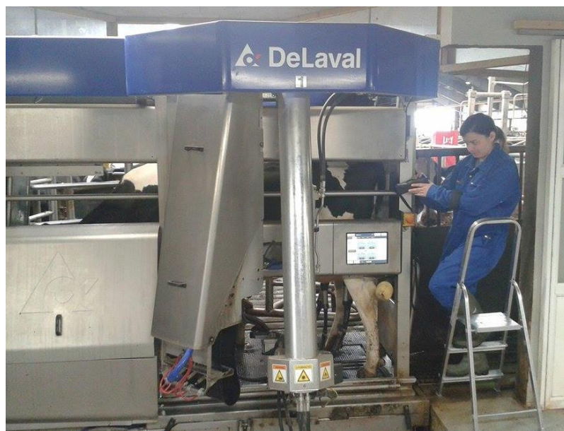
Figure 2: methane measurement in an AMS with LMD
