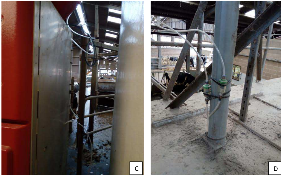
Picture 2. Inlet tube that sample the air in the bin rare (A). Air sampled through the instrument by an integral pump between the gas inlet port and analyser (B, C); Inline combined particle filter with water separator (D)
