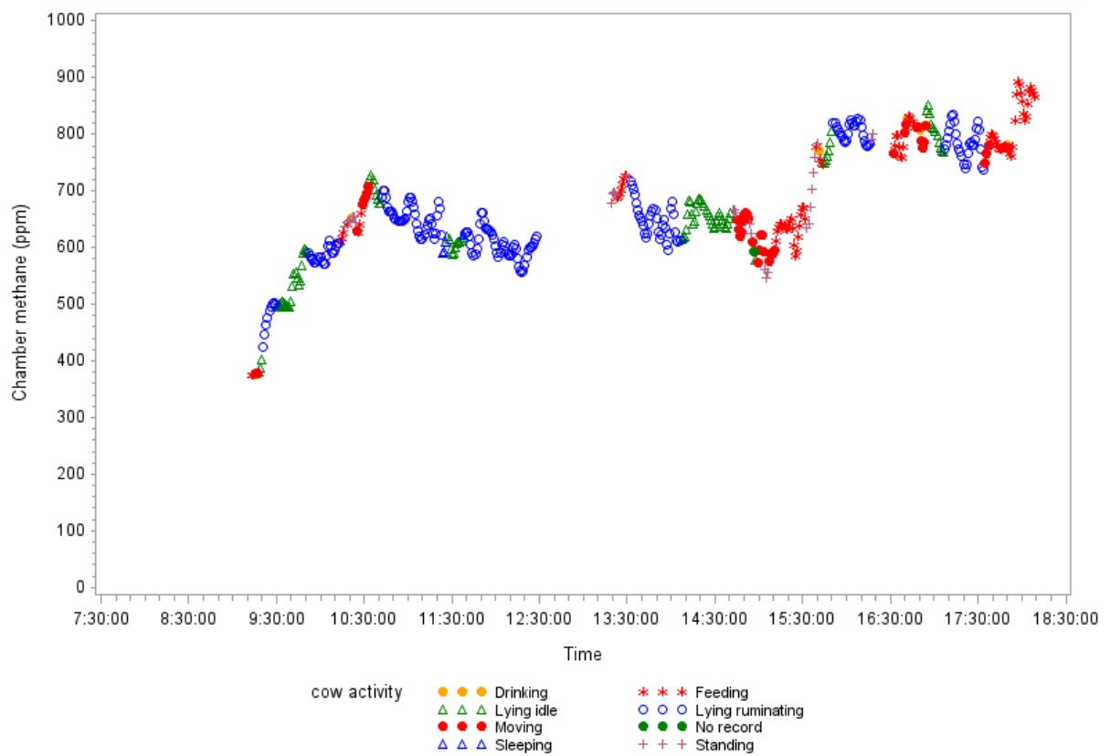
Fig. 8: Chamber methane in chamber 2, coloured by cow activity.
